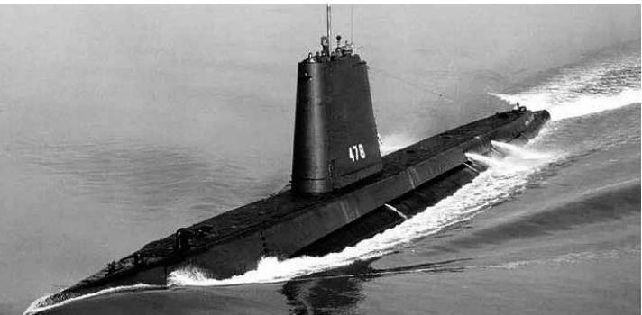
As part of a 1957 overhaul, Cutlass was fitted with a new fiberglass high sail, also known as a North Atlantic sail.
